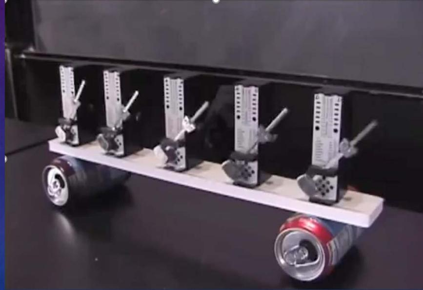
Phase synchronization of bidirectionally coupled metronomes at 176 beats per minute
